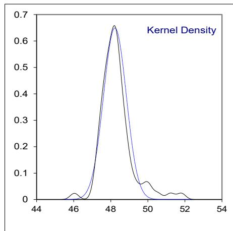
Determination of Kinematic Viscosity Stabinger at 50 °C on sample #22100; results in mm<sup>2</sup>/s
