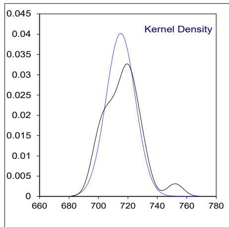
Determination of Kinematic Viscosity Stabinger at 100 °C on sample #22100; results in mm<sup>2</sup>/s
