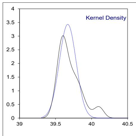
Determination of Kinematic Viscosity at 50 °C on sample #22100; results in mm<sup>2</sup>/s
