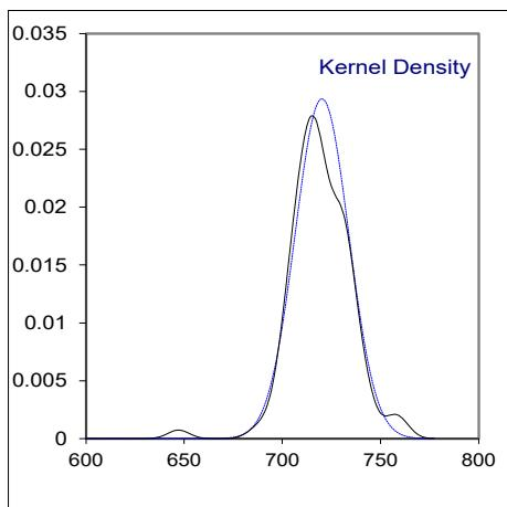
Determination of Kinematic Viscosity at 100 °C on sample #22100; results in mm<sup>2</sup>/s
