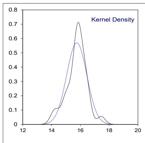
Determination of Density at 15 °C on sample #22100; results in kg/m<sup>3</sup>
